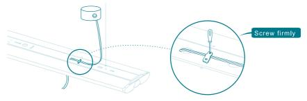
Insert the power cable into white terminal block.(Please refer to installation guide of Surface-Mounted type step 3.)
