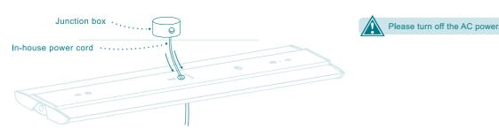
Insert the in-house power cord into white terminal block which fixed inside the luminaire.
