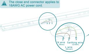
nsert the 18 AWG AC power cord into the close end connector and press the end of the connector by tools such as crimping pinchers to insure the wires are not fallin
