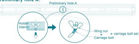
Pass the in-house power cord through the outlet hole of the holder. Put the carriage bolt set to T-accessory's ceiling lock hole a.
